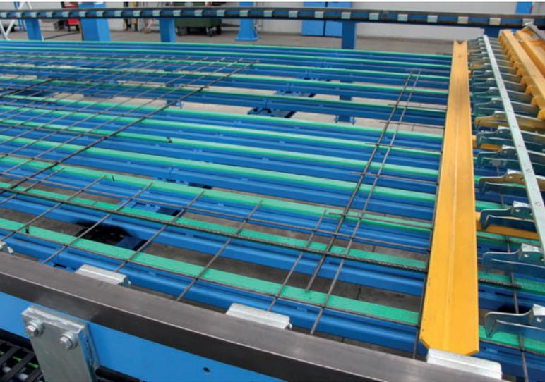
Reinforcement mesh can be produced automatically with openings for window and door spaces. No further manual cutting is required. This leads to major savings in raw material and manpower costs.
